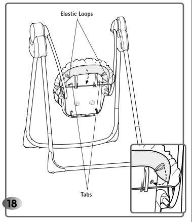
• From behind the seat, fit the pad elastic loops to the tabs on the seat back.
